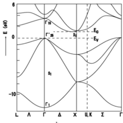
Band spectrum of silicon along special directions
