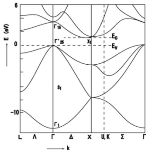
Band spectrum of silicon along special directions
