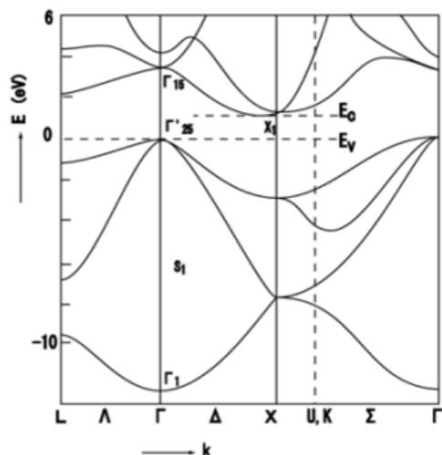
Band spectrum of silicon along special directions
